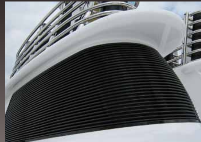
▲ Hingeable louver with lamella intergrated unlocking system
